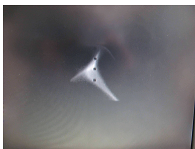
Figure 2. Proton beam profile observed by the KBr viewer plate at the downstream of the NEOMAFIOS. The intensity was 10 \mu\text{A} at 15 kV extraction voltage.
