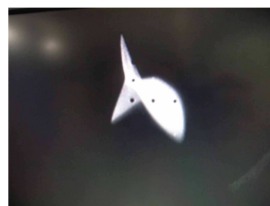
Figure 3. ^4\text{He}^{2+} beam profile observed by the \text{BaF}_2 viewer plate at the downstream of the NEOMAFIOS. The intensity was 200 \mu\text{A} at 15 kV extraction voltage.
